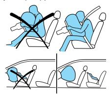
All occupants of the vehicle, including the driver, should always properly wear their safety belts, even when an air bag SRS is provided.
